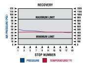
Brake: 14 1/2" x 10" Meritor® W Brake Axle Load: 26.000 lb AL Factor: 210 Normal Friction: .431 F Hot Friction: .423 F
